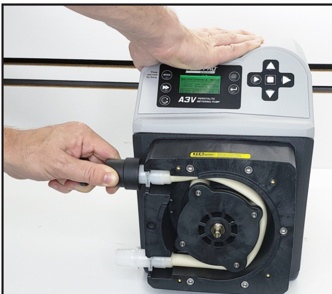
Continue to follow rotation of rotor while directing tube into pump head. At this point, you may need to pull Tube Installation Tool to stretch tubing into position. Let rotor spin a few rotations while pulling Installation tool so fitting can be properly installed.
