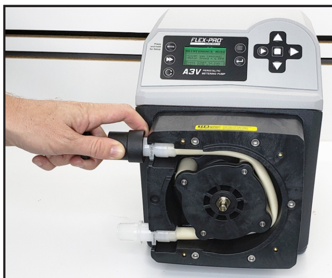
Continue to pull Tube Installation Tool to allow enough room to slide discharge fitting into pump head tongue and groove. Once discharge fitting is secured in pump head, stop pump by pressing STOP button. Replace pump head cover. Pump will ask you if the tube was replaced, select yes. Pump will then ask if you would like to reset Tube Hours, select yes. Tube Hours will reset to zero.
