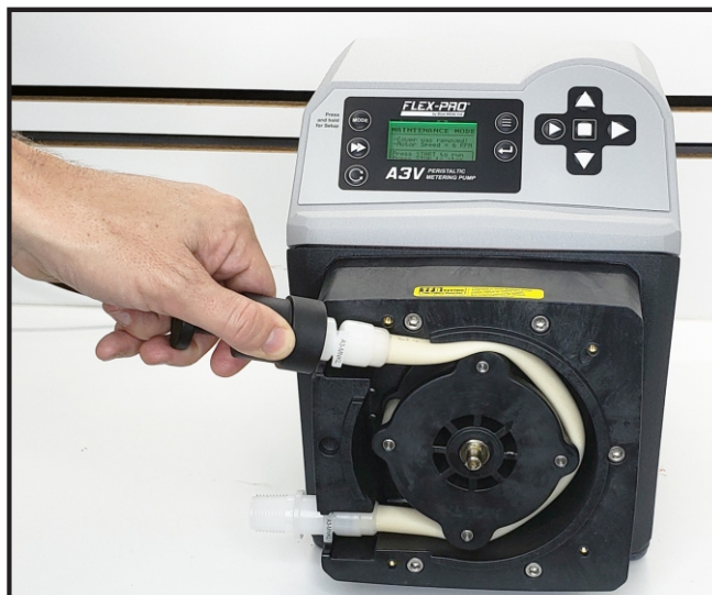
Introduce tubing into pump head while the rotor is rotating. Avoid using fingers to guide the tubing. Stop pump at anytime by pressing STOP button. Start pump by pressing START button.
