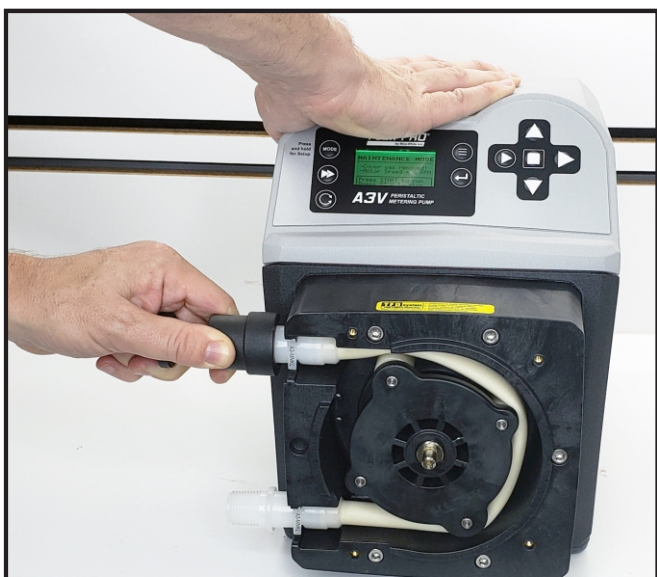
Continue to follow rotation of rotor while directing tube into pump head. At this point, you may need to pull Tube Installation Tool to stretch tubing into position. Let rotor spin a few rotations while pulling Installation tool so fitting can be properly installed.
