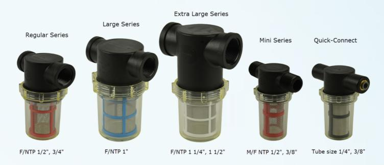
In-line Strainer Series, 20% Glass filled polypropylene body with EPDM gasket and Clear bowl. A selection of 20, 50 or 80 mesh Stainless Steel Screen prevents from dirt and other industrial water debris to damage the probes, solenoid valves, re-circulation pumps, as well as protecting the entire piping assembly. Applications: Pool and Spa, Cooling towers, Industrial water applications.
