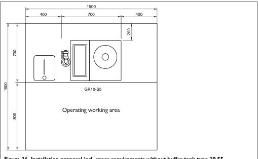
Figure 16, Installation proposal incl. space requirements without buffer tank type 10-S5
