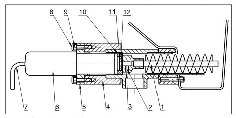
Figure 34, Dosing motor with dosing screw
