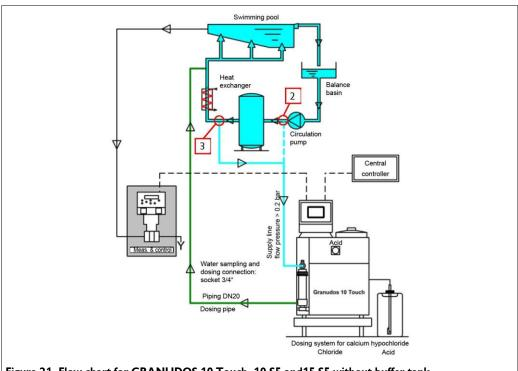
Figure 21, Flow chart for GRANUDOS 10-Touch, 10-S5 and 15-S5 without buffer tank
