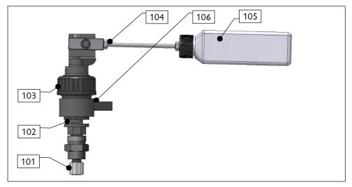
Figure 39, Floater control valve for GRANUDOS 15, complete
