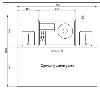
Figure 15, Installation proposal incl. space requirements without buffer tank type CPR Touch XL and Touch
