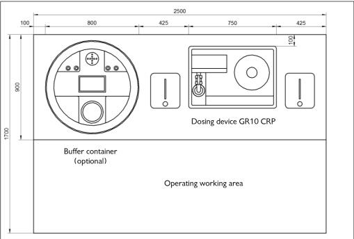
Figure 18, Installation proposal incl. space requirements without buffer tank type CPR Touch XL
