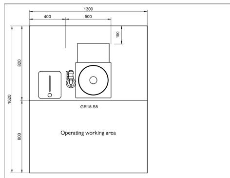
Figure 17, Installation proposal incl. space requirements without buffer tank type 15-S5
