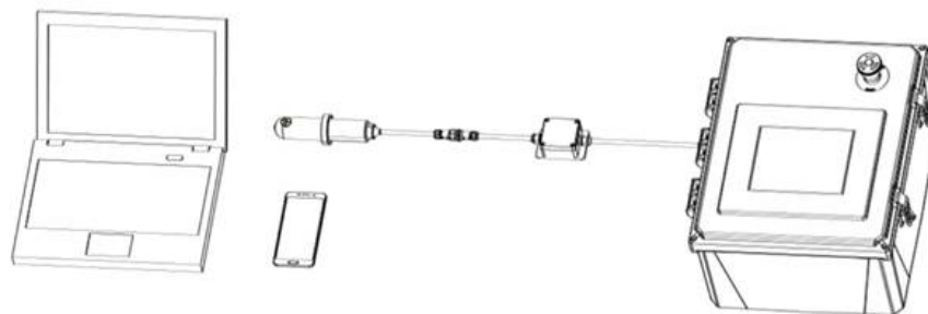
Figure 5. Bluetooth connection to HM-500 Series sensor
