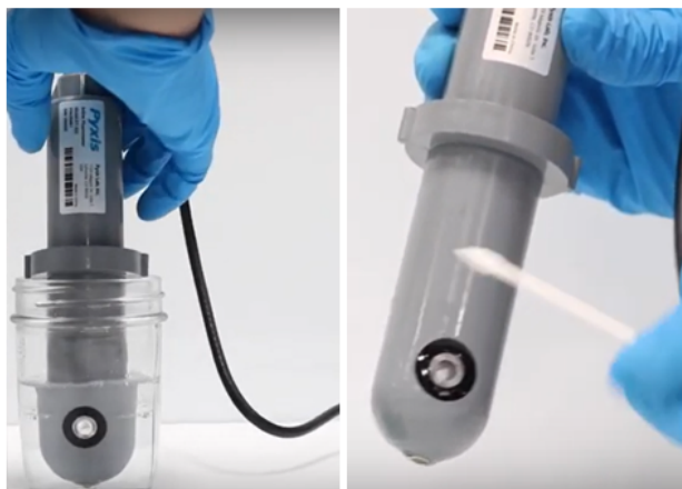
Figure 19. Cleaning of HM-500 Series Sensor
